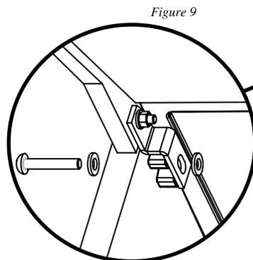
4. Attach the **Right Mounting Bracket** to the top foot on the Apple & Fruit Crusher with the **1½" Machine Screw, two Flat Washers & Hex Locking Nut (G)**.
