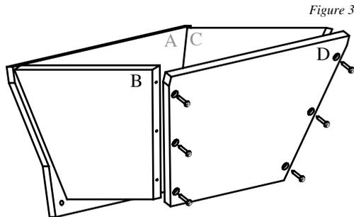
7. Align the pilot holes on the **Right Side Board (C)** with the through holes on the **Front Board (D)**.
