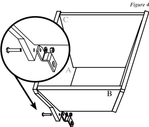
9. Attach the **Left Mounting Bracket (E)** to the **Back Board (A)** with the **1" Machine Screw, Washer and Hex Locking Nut (F)**. *FIGURE 4*
