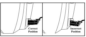
Fig. J For proper connection, the magnetic plug end must be parallel with the countertop.
