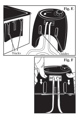
Important: The magnetic cord was designed to detach easily from the fryer. As a result, if it is bumped or touched during use it could possibly detach causing the unit to stop heating. Avoid contact with cord during operation. If contact occurs, verify that the cord is still properly connected.
