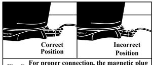
Fig. C For proper connection, the magnetic plug end must be parallel with the countertop.
