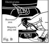
When properly aligned, the plug will magnetically attach itself to the appliance. For proper connection, the magnetic plug end must be parallel with the countertop (Fig. C).
