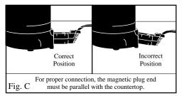
Important: The magnetic cord was designed to detach easily from the fryer. As a result, if it is bumped or touched during use it could possibly detach causing the unit to stop heating. Avoid contact with cord during operation. If contact occurs, verify that the cord is still properly connected.
