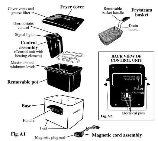
can also occur if using solid fat or older oil that has become thick. Should the unit shut off, unplug and allow the unit to cool. Correct the cause of overheating. Then with the tip of a pen, press the red RESET button on the back of the control unit (Fig. A2). The unit will not operate until it is reset.
